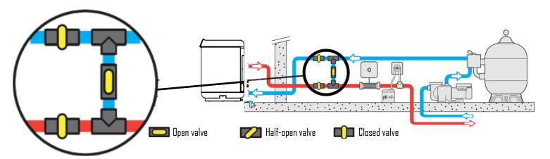
Unscrew the junctions to evacuate all the water contained in the HP.
