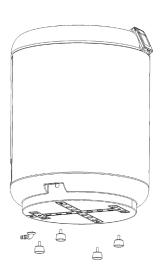
The Ottimo HP has four feet and a condensate extraction nozzle included with the product. the condensate extraction nozzle and the four feet must be attached before installing the machine, using the described methode in the figure above.
