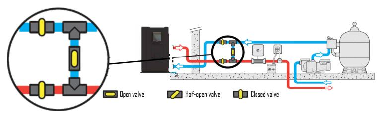
Unscrew the junctions to evacuate all the water contained in the HP.
