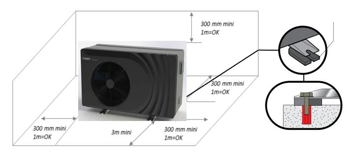
The HP must be installed and maintained on a fixed and solid basis, with the skids placed under the feet.
