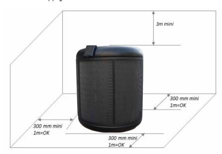
The HP must be installed and maintained on a fixed and solid basis, with the skids placed under the feet.
