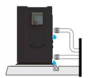
Reconnect and slightly tighten the junctions by hand to prevent the introduction of foreign objects into the HP
